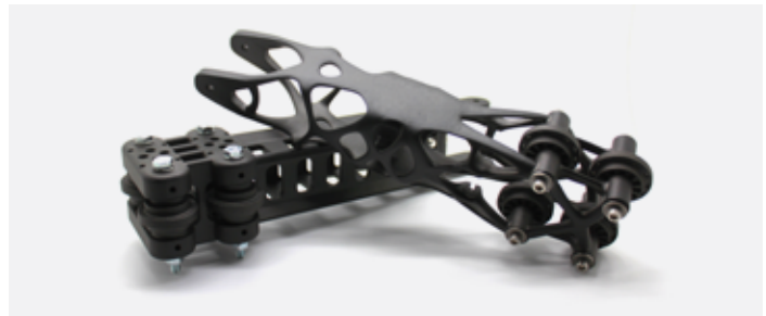
This robot arm was printed using HP Multi Jet Fusion technology with PA 12 (Nylon 12) material and a steel gray (formerly carbon gray) finish.
