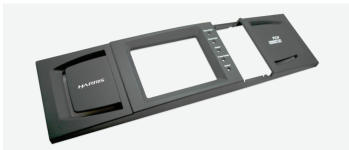
This computer housing was made using cast urethane with cast-in custom color with UABS 83 (PX224) material and post-process pad printing.
