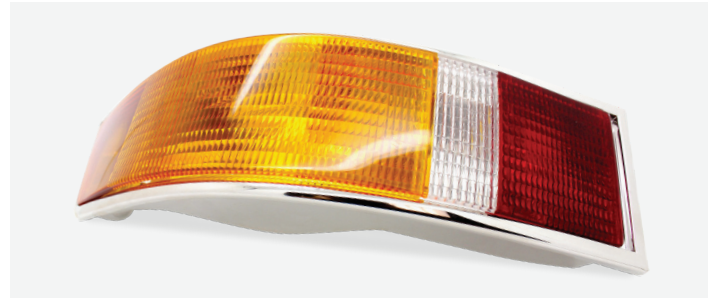
This rear auto light lens was made using cast urethane with cast-in custom colors and a Clear Uoptic 3 (multiprocess cast process) material. The rear light bucket used UABS 83 material and cast urethane with post-process chrome plating.
