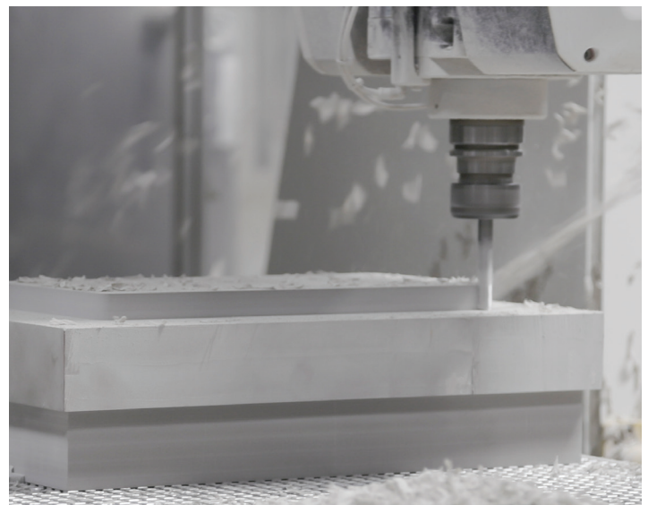
CNC machining the production tooling from CAD data
