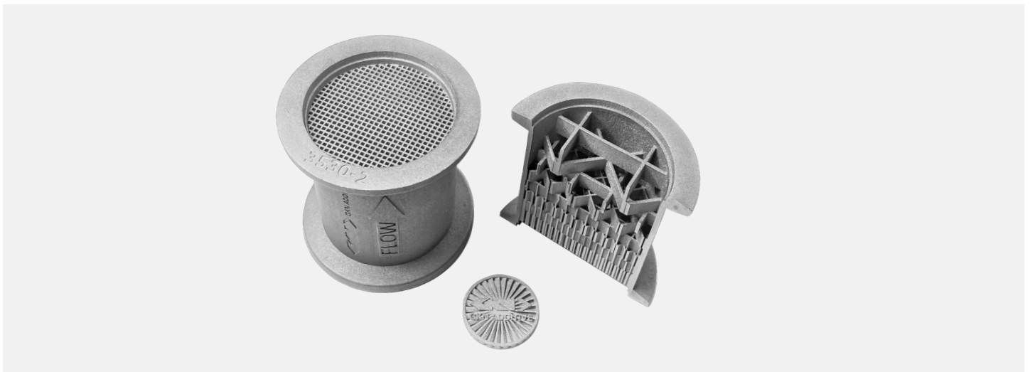
This complex static mix element shows geometries based on static mixers. Note the inner cavities in the blades and the ring channel, which can be produced reproducibly in large quantities using binder jetting technology.
