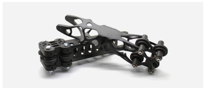
This robot arm was printed using HP Multi Jet Fusion technology with PA 12 (Nylon 12) material and a carbon gray finish.
