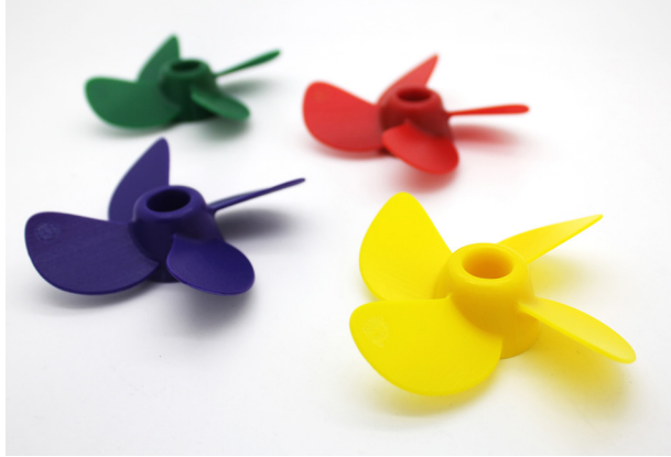
Figure 4: PolyJet is a widely used rapid prototyping process, and was the first to provide over-molding capabilities to engineers.
